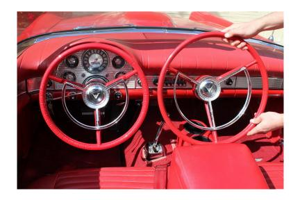
Here's a side-by-side comparison of an original 1957 Thunderbird steering wheel next to the installed 3600SM steering wheel.
