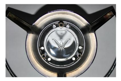
Next install the new Thunderbird medallion in the horn ring casting. There is a small notch at the top of the medallion which mates with a corresponding key on the casting. (You can see the notch at the top center of the photo). Install the conical metal piece over the medallion and then reinstall the hub assembly, being careful to align the rubber insulator and spacers. Tighten the three Phillips screws in sequence until the hub assembly is secure.
