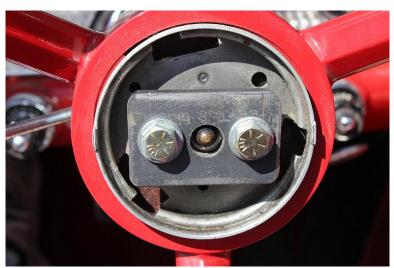
Here is the steering wheel puller in place, ready to do its duty. Each hex bolt is gradually tightened using a 1/2" socket wrench. Once one bolt feels tight, move to the other. Eventually the steering wheel will be loosened on the shaft and can be easily removed just by pulling it toward you.
