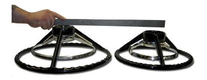
The 3600SM steering wheel is also 1" less in height than the standard thunderbird steering wheel. This combination provides extra room for the driver, almost like pushing the seat a little farther back.
