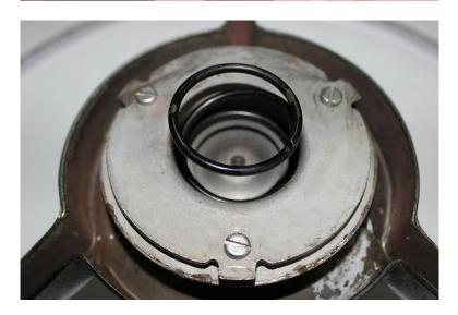
The back of the original T-Bird horn ring shows the horn ring spring. This part, CASCO No. 13A807, is not included with the 3600SM smaller steering wheel, so be sure to order one from CASCO when you buy the new steering wheel. This way you can store the original steering wheel as an intact unit, complete with center medallion and horn ring spring.
