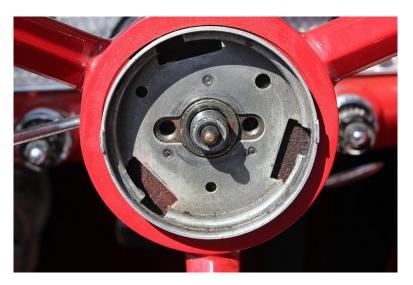
Here is a view of the original steering wheel hub after the lock nut was removed. You can clearly see the horn button contact in this photo.
