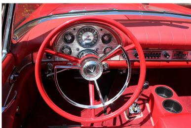
It is now time to remove the original T-Bird steering wheel. First, park the car with the wheels pointed straight ahead and disconnect the negative battery cable. Remove the horn ring by firmly and evenly pressing inward while simultaneously giving the ring a twist to the left. When it gets to the position shown in the photo, it should lift right off.
