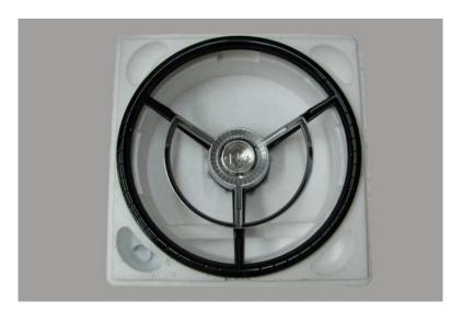
The 3600SM steering wheel arrives well packaged in a Styrofoam container, complete with horn ring and a generic center medallion. The small half-round clip shown in the lower left corner of the container gets installed on the back of the wheel hub and is used to automatically cancel the turn signals. If your interior happens to be black, you can install your new wheel. Otherwise, the wheel must first be repainted in the correct color.
