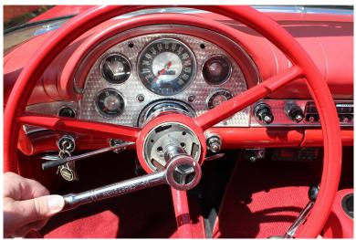
Remove the nut with a 15/16" socket wrench and extension, being careful not to scratch the paint on the steering wheel.
