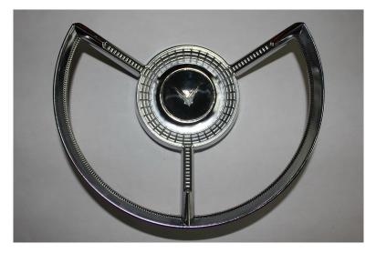
Flip over the horn ring and it should look like this photo. Other than the smaller size, the only thing that distinguishes the 3600SM horn ring from some originals is that it lacks the "Ford Master Guide Power Steering" legend under the hub. Ironically, the smaller steering wheel is probably only appropriate for those cars that actually HAVE power steering, but basing the repro horn ring on a manual steering car likely avoids a Ford licensing issue.
