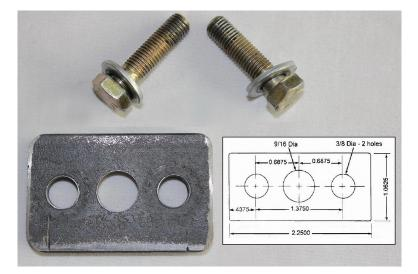
This is the steering wheel puller that was made from a diagram published in Issue 10, October 1997 of CASCO's ThunderEnlightening newsletter. A piece of ½" thick steel bar stock and a drill press are used to make the custom puller. The large center hole is critical, because it enables the horn button wire to poke through without being damaged. The two hex bolts are 5/16-24 (fine thread), 1-1/4" long.
