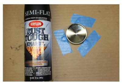
The other part of the horn ring assembly is a round conical-shaped trim piece that is mounted directly behind the center emblem. If your T-Bird is a 1956, the supplied silver color is correct. The example car was a 1957, so it was necessary to paint this piece black. Carefully scuff the surface with steel wool, clean it with solvent, primed it and then painted it. Semi-flat black spray paint from a rattle can works fine.
