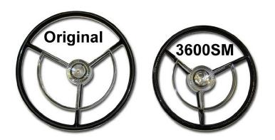
The 3600SM smaller steering wheel is a solution for those 1956/57 T-Bird owners who desire some extra wiggle room from the driver's position. The 3600SM is a scaled down reproduction steering wheel with matching horn ring that is 2" less in diameter than a stock 1956/57 Thunderbird steering wheel.
