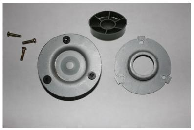
If you separate the components of horn ring hub assembly, you will find a large rubber insulating spacer as well as three rubber spacers. These serve to isolate the two circular metal pieces of the hub. This isolation is necessary for the proper functioning of the horn relay circuitry.
