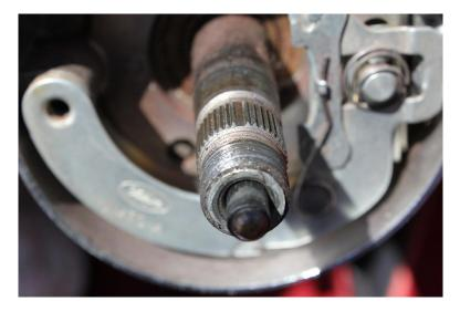
This close-up view of the steering wheel shaft shows that the shaft is keyed with a wider groove at the top of the assembly. This wide groove mates with a corresponding wider key on the steering wheel hub. The wheel can only fit on the shaft one way.
