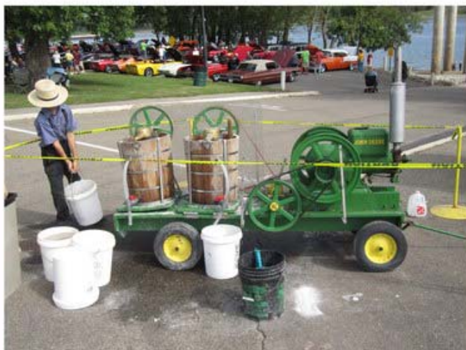
Ice cream maker powered by John Deere "hit & miss" engine
