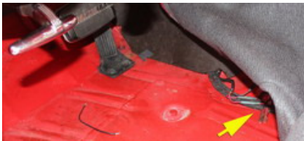
Connections to Neutral Safety/Backup Switch
